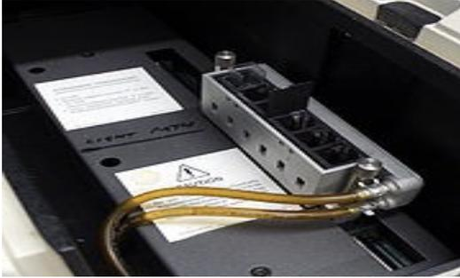
Temperature-controlled [cuvette](#) holder in a spectrophotometer.
