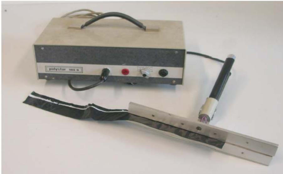
*Fig. 2: A heat paste machine “Polystar 100 G” used for producing biodegradable laterals*
