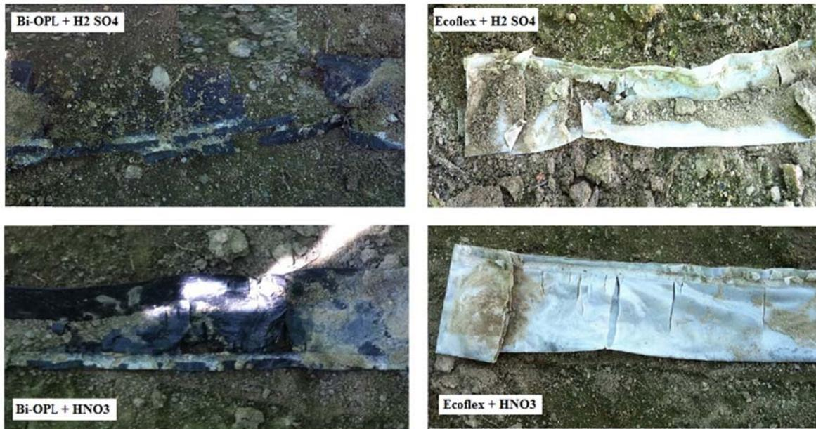
Fig. 5: The bioplastics degradation after the exposure time at field
