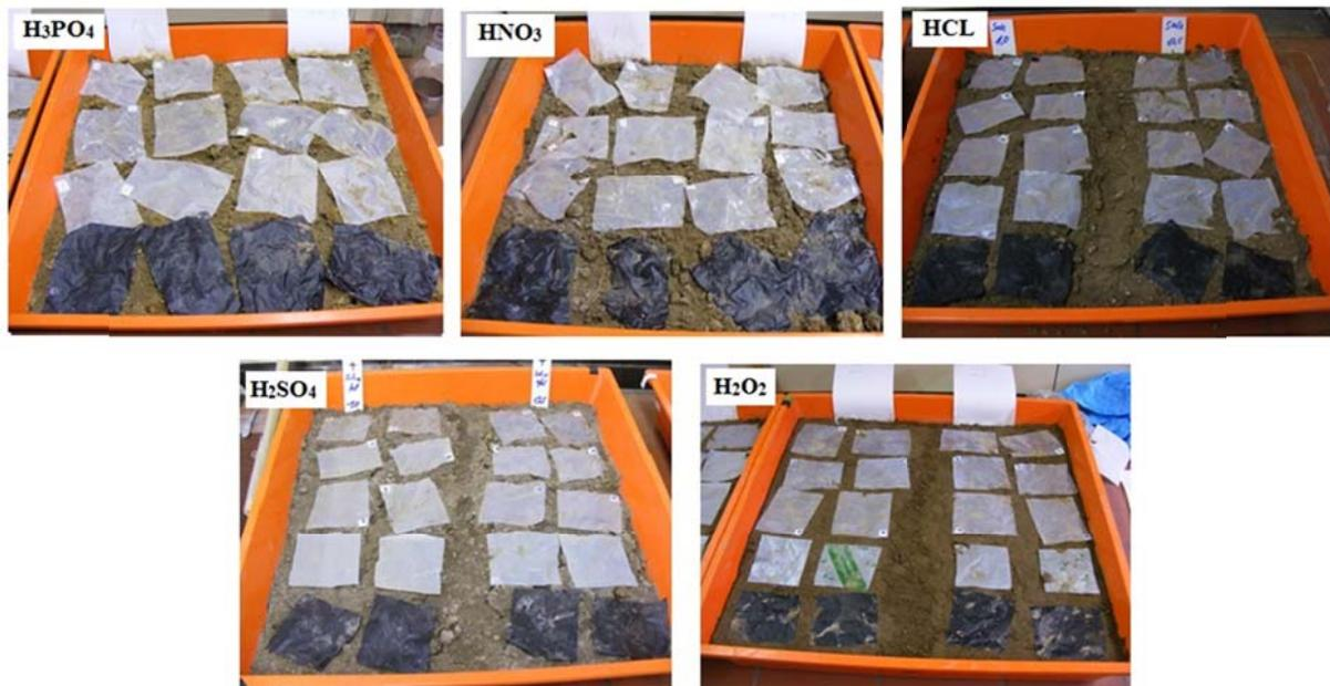
*Fig. 4: The bioplastics degradation after the exposure time at laboratory.*
