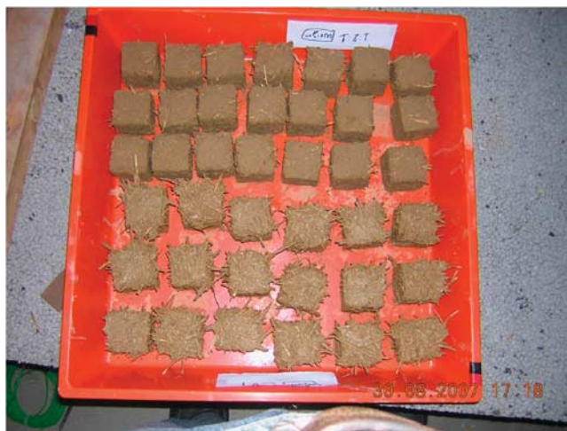
Figure 1: Samples prepared for drying test and water absorption.
