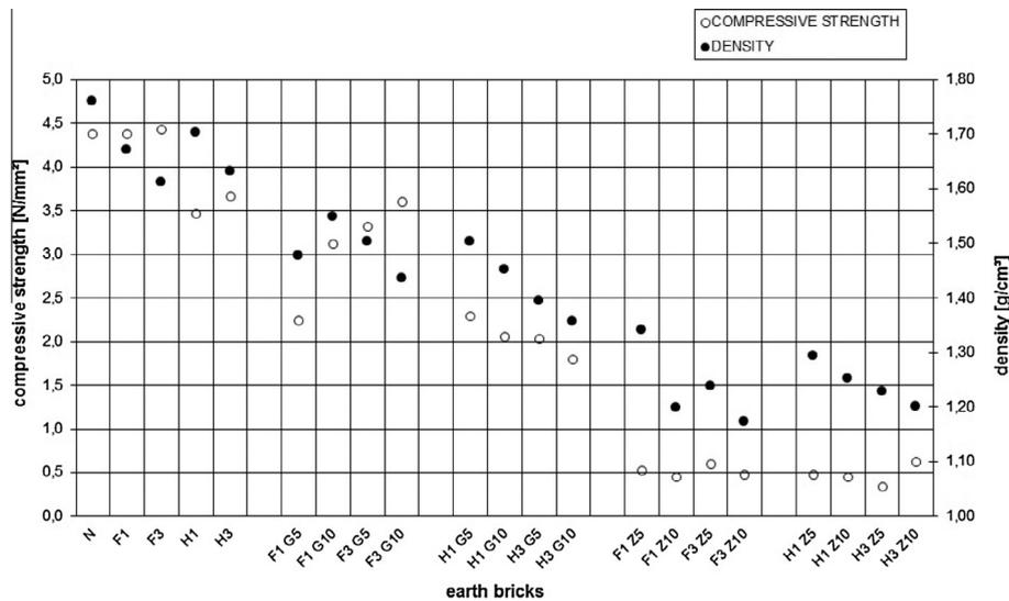
Fig. 9. Influence of density on compression strength of earth bricks.
