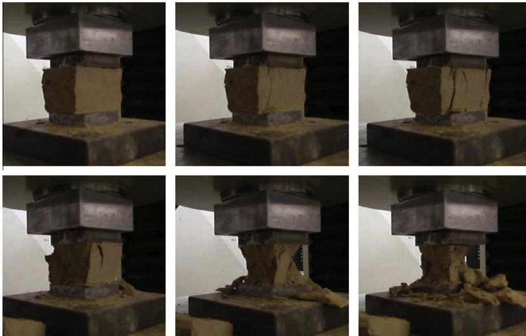
**Fig. 4.** Breaking process of earth bricks without additives.
