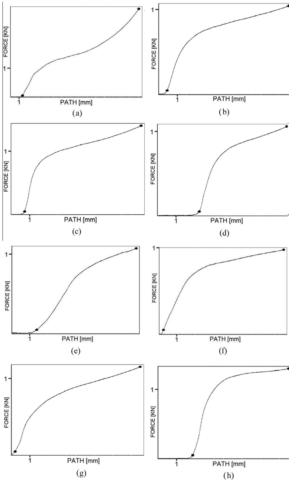
**Fig. 8.** Force–path diagrams of bricks made from cement mixtures and other materials, (a) flax 1% and cement 5%, (b) flax 1% and cement 10%, (c) flax 3% and cement 5%, (d) flax 3% and cement 10%, (e) hemp 1% and cement 5%, (f) hemp 1% and cement 10%, (g) hemp 3% and cement 5%, (h) hemp 3% and cement 10%.
