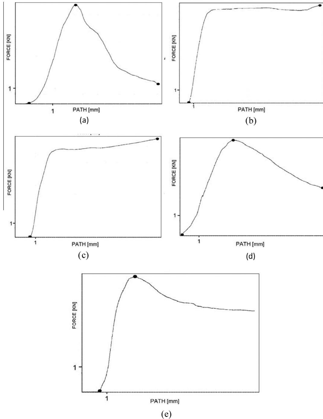
**Fig. 6.** Force–path diagrams of bricks with different fibers type and contents, (a) without additives, (b) flax 1%, (c) flax 3%, (d) hemp 1%, (e) hemp 3%.
