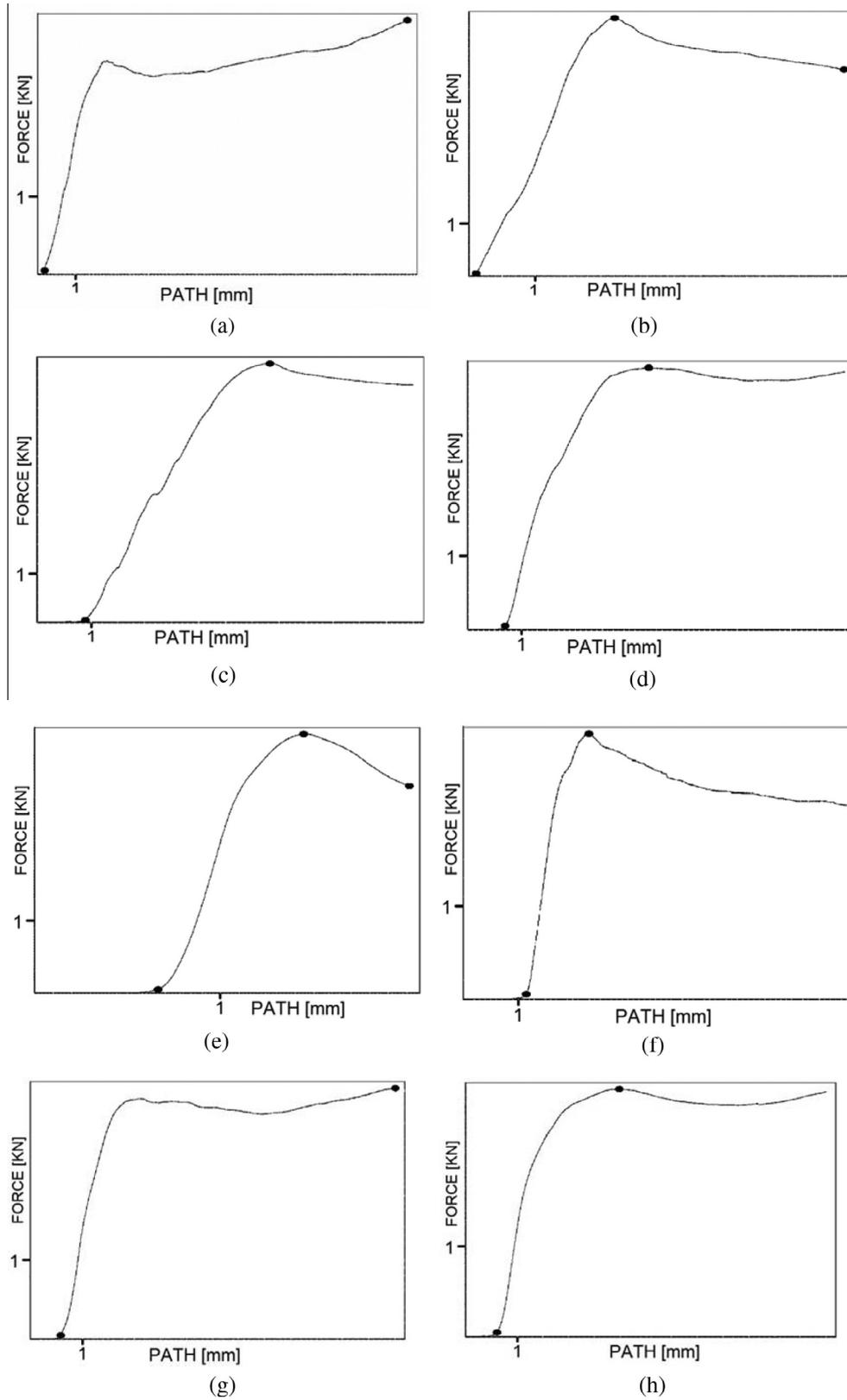
**Fig. 7.** Force–path diagrams of bricks made from gypsum mixtures and other materials. (a) flax 1% and gypsum 5%, (b) flax 1% and gypsum 10%, (c) flax 3% and gypsum 5%, (d) flax 3% and gypsum 10%, (e) hemp 1% and gypsum 5%, (f) hemp 1% and gypsum 10%, (g) hemp 3% and gypsum 5%, (h) hemp 3% and gypsum 10%.
