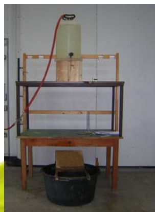
Fig.3. Erosion test set up
