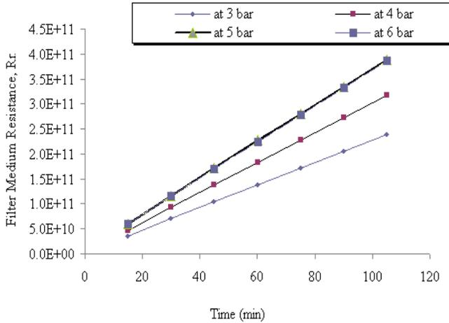
Fig. (6) : Effect of UF operational pressure on the filter medium resistance ( $R_m$ ) as a function of time during milk concentration.
