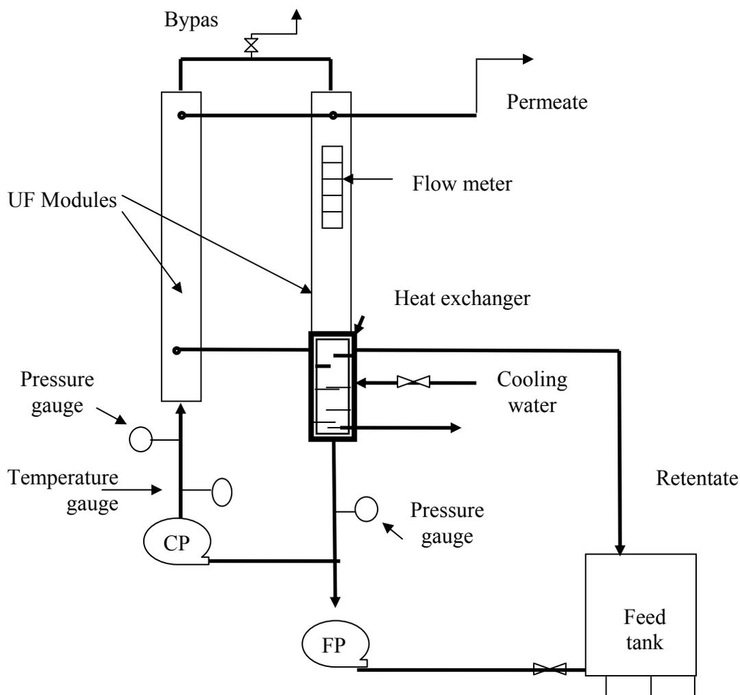
*Fig 1.* Schematic of the experimental setup.
