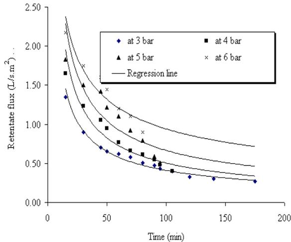
Figure (2) Retentate flux at different operational pressures of UF process.
