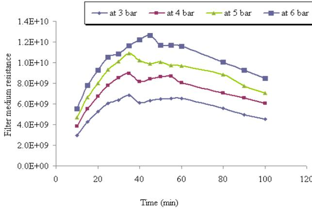
Fig. (7) : Filter medium resistance during cleaning process of UF at different operational pressures.
