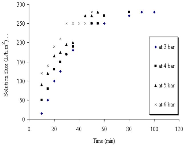
Figure (4) :Flux recovery during cleaning at different operational pressures.
