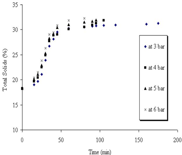
Figure (5) :Milk concentration at different operational pressures.
