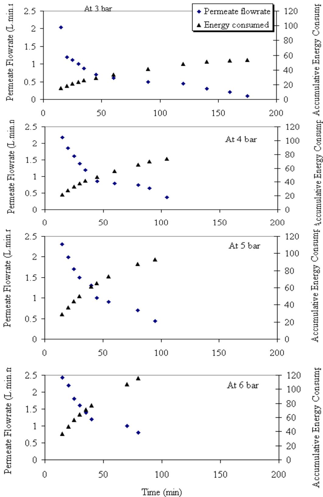
Fig. (9) :Permeate flowrate and accumulative energy consumption at different operational pressuresUF milk concentration.
