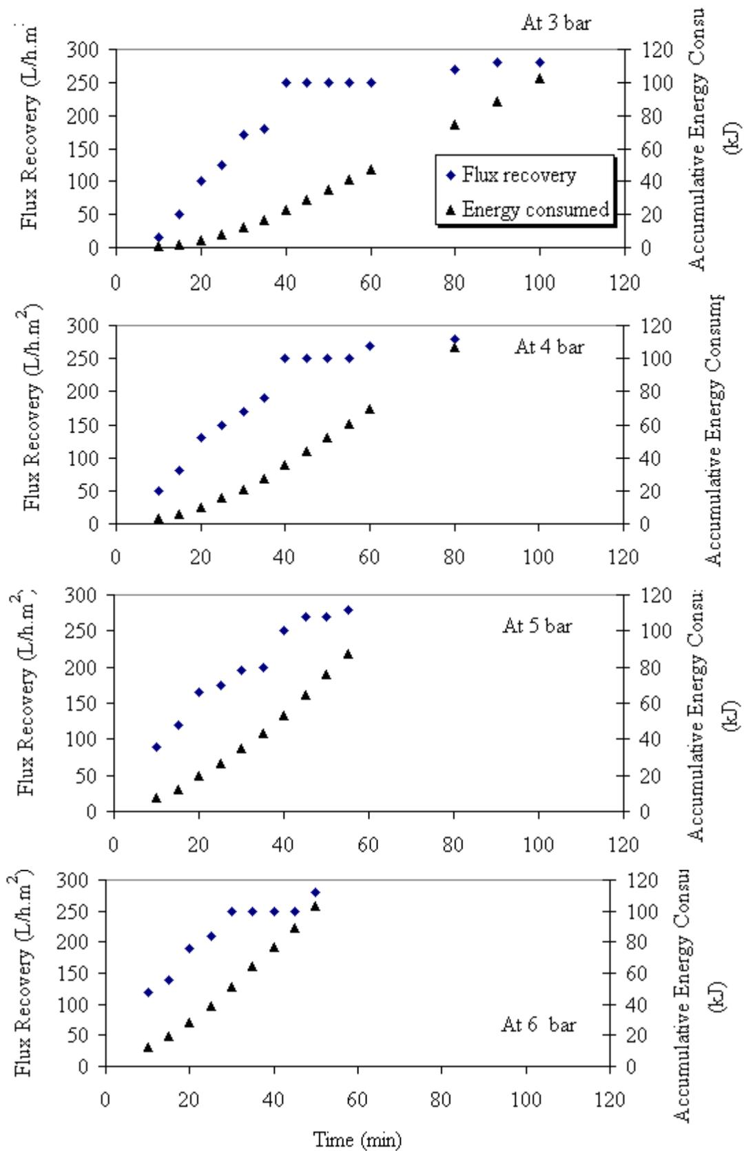
Fig. (10) :Flux recovery and accumulative energy consumption at different operational pressures during UF cleaning.
