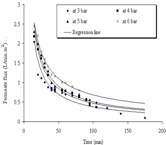
Figure (3) Permeate flux at different operational pressures of UF process.
