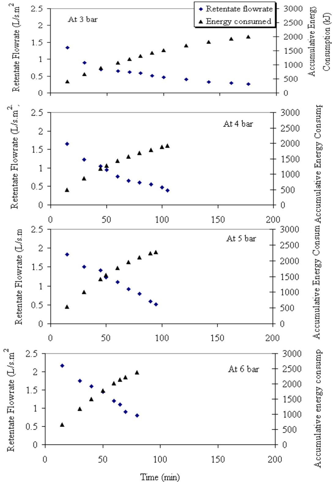
Fig. (8) .Retentate flowrate and accumulative energy consumption at different operational pressures during UF milk concentration.
