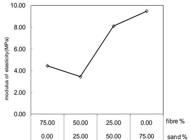
**Fig 9.** Modulus of elasticity for plaster reinforced with wood shavings fibers
