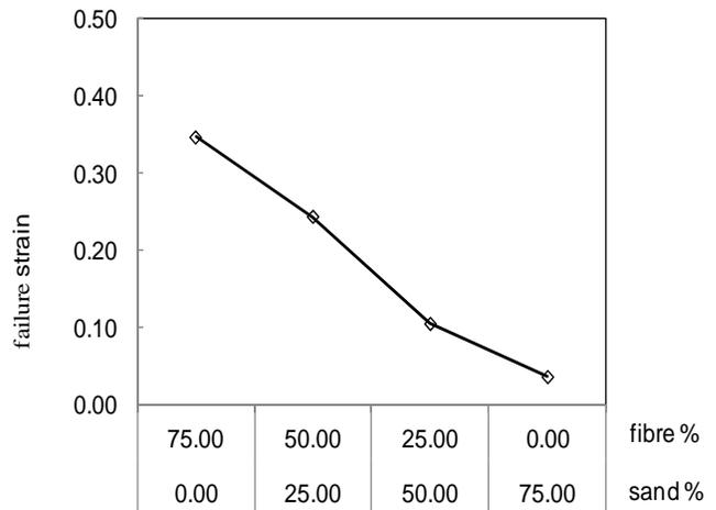
**Fig 8.** Failure strain for plaster reinforced with barley straw fibers
