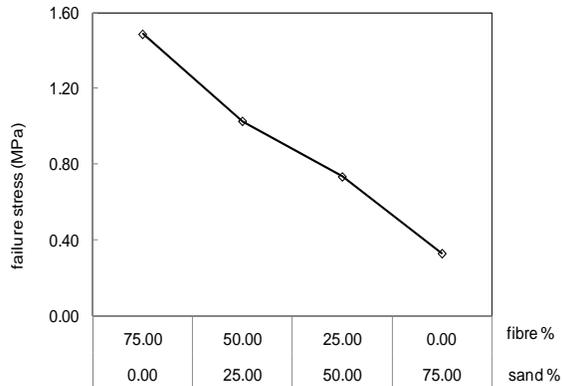
**Fig 3.** Failure stress for plaster reinforced with wood shavings fibers
