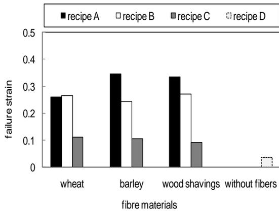
**Fig 13.** Failure strain for the different treatments
