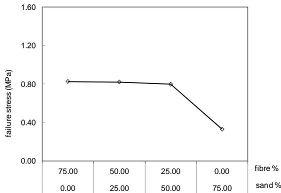
**Fig 4.** Failure stress for plaster reinforced with wheat straw fibers
