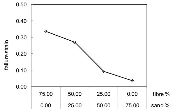
**Fig 6.** Failure strain for plaster reinforced with wood shavings fibers
