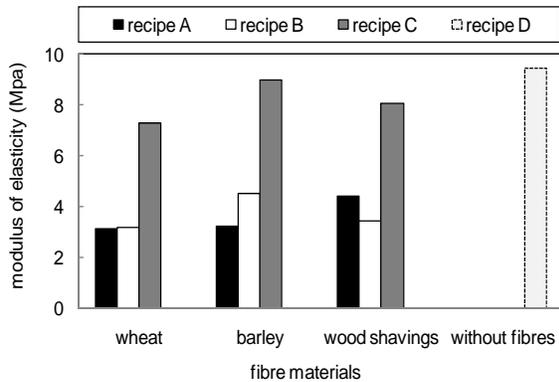
**Fig14.** Modulus of elasticity for the different treatments at failure condition
