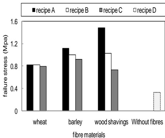
**Fig 12.** Failure stresses for the different treatments
