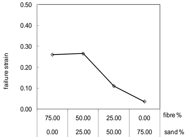
**Fig 7.** Failure strain for plaster reinforced with wheat straw fibers
