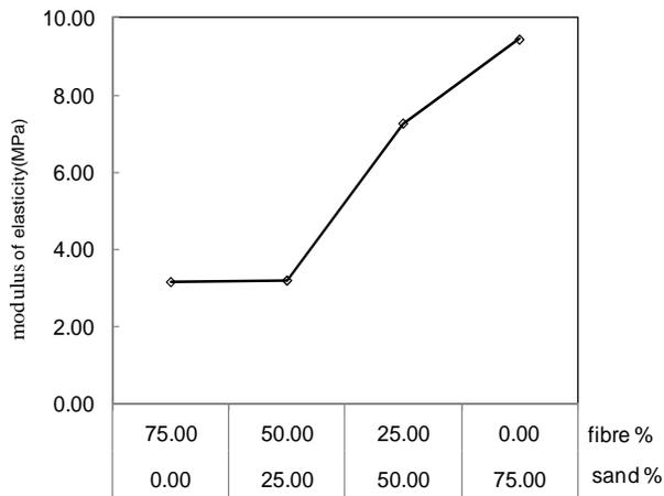
**Fig 11.** Modulus of elasticity for plaster reinforced with wheat straw fibers
