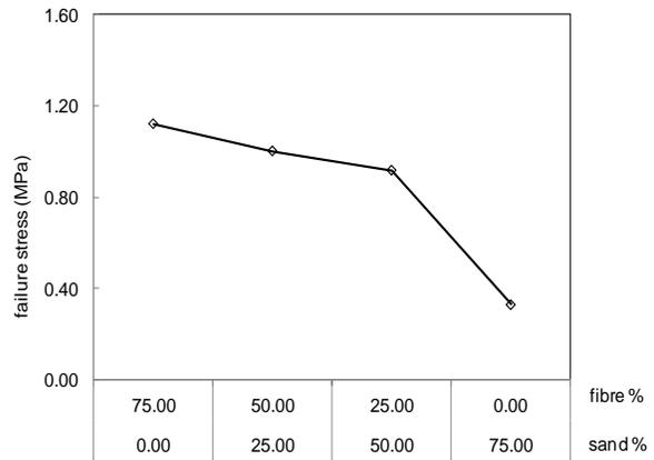
**Fig 5.** Failure stress for plaster reinforced by barley straw fibers
