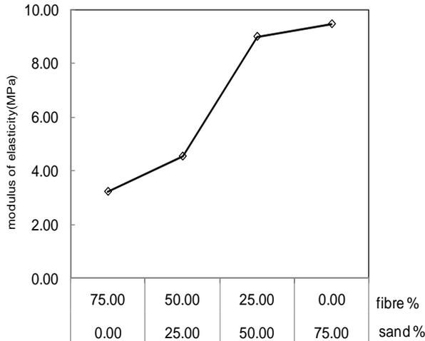
**Fig 10.** Modulus of elasticity for plaster reinforced with barley straw fibers
